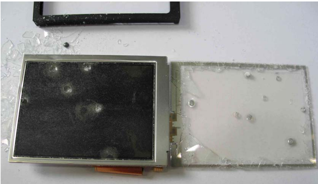
Figure 3 – Close-up view on the display, touch panel and rubber gasket
