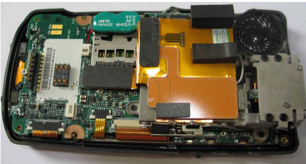
Figure 4 – Inside view showing no penetration of glass dust
